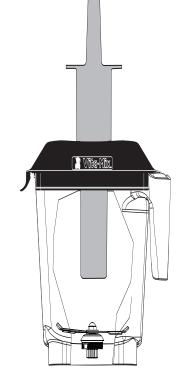
\*NOTE: Accelerator Tools have a small step on them. The step prevents the Accelerator Tool from coming into contact with the blades in Vita-Mix polycarbonate containers. Accelerator Tool cannot be used with a one piece non-latching lid.
